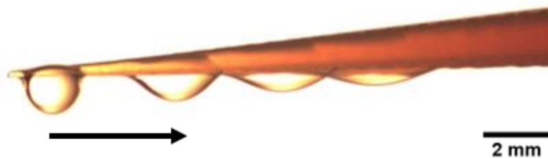
FIGURE 1 – Superposition of successive pictures emphasizing the motion of a large droplet on a 3d printed conical structure. The motion is shown at time t = 0s, 2s, 7s and 14s .
