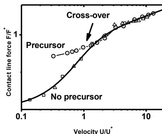
Figure 1: Illustration of the onset of the **precursor** film in advancing contact line motion - **MDS**. **Density distribution** (liquid is shown in dark colour) in complete wetting case and the out-of-balance **contact line force**  $F/F^* = \gamma_{GS} - \gamma_{LS} - \gamma \cos \theta_c$  as a function of normalized velocity  $U/U^*$  in complete wetting (static angle  $\theta_S = 0$ , precursor present) and incomplete wetting (static angle  $\theta_S > 0$ , no precursor) cases.
