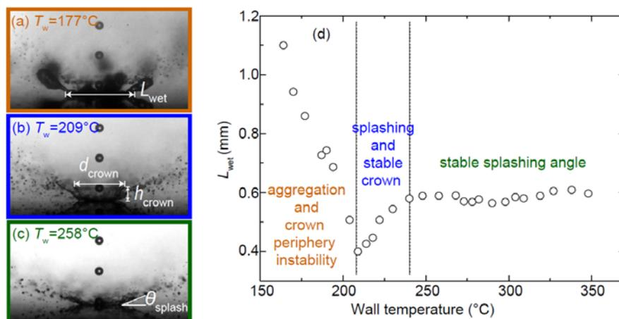
Figure 1 The typical steady-state hydrodynamic patterns for the regime of (a) the wetting length, (b) the stable crown and (c) the splashing angle. (d) shows the wetting length vs the surface temperature.
